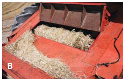
Hemp fibre clogging the cutting bar (A) and combine paddles (B, swathed)
