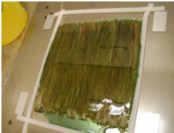
b: Epoxy added to the lay up
