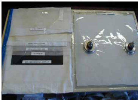
a1: Lay up for autoclave consolidation
