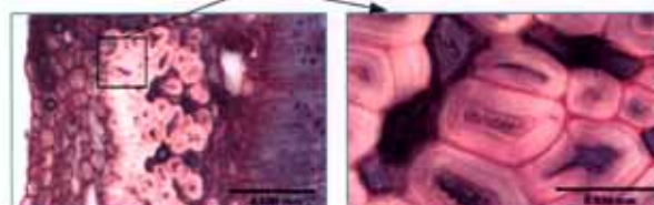
Light microscopy image of Ruthenium red stained hemp stem section. Pectin is stained red.
