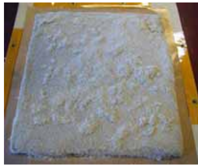
b1: Lay up for press consolidation
