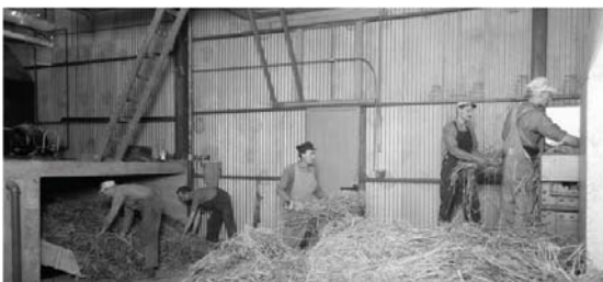
2022-1 Ohlwa Vista Hemp Plant (This is probably Imperial Linen) 0.1934 It is delivered to the machine where an automatic chain conveyor feeds it to the breaking arms at the rate of two or three tons per hour. The hurds are broken into fine pieces which drop into the hopper, from where they are delivered by blower to a baler or to truck for freight care for loose shipment. The fiber comes from the other end of the machine ready for bailing.
