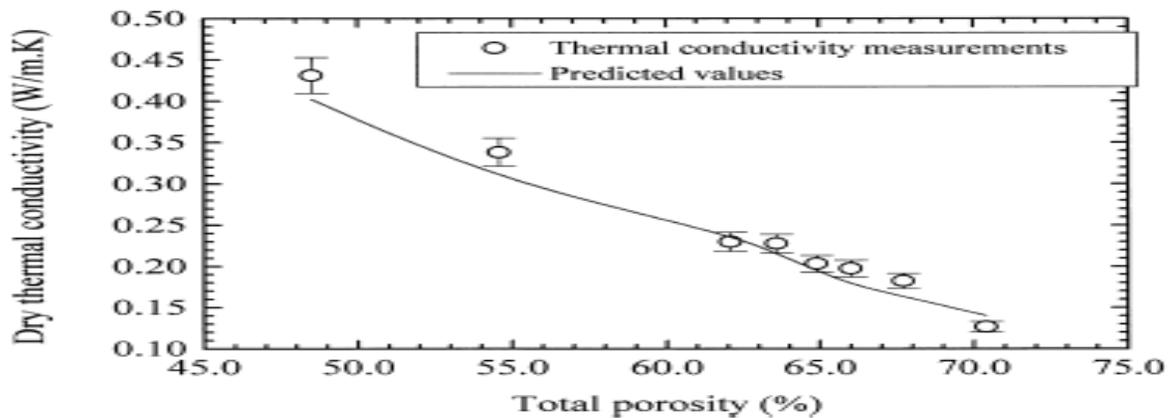
**Figure 1: The effect of porosity.** Source: Bouguerra (1998).
